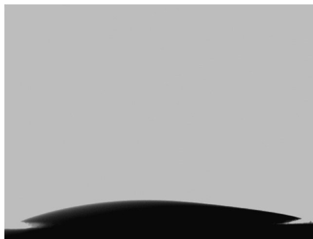
Fig. 5. Water contact angle measurement of \text{Fe}_2\text{O}_3 thin film.
